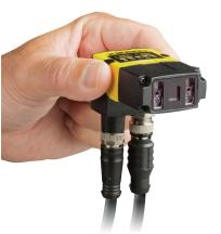
DataMan 150/260 barcode readers with ImageMax technology is an ideal solution for reading wide range of hard to read 1-D linear and 2-D matrix codes in even the most challenging environments in industries, such as automotive, electronics, packaging, and logistics.
